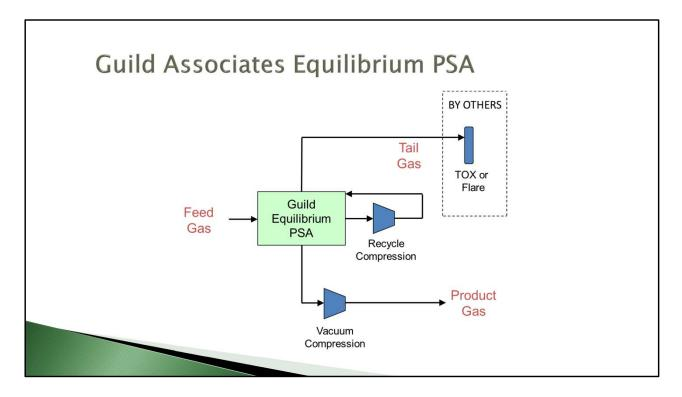
Details of the process flow diagram:
