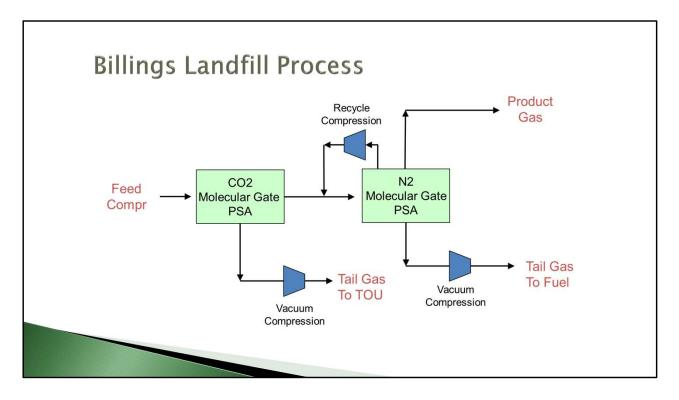
Similar to previous process flow diagrams, this system incorporated a Molecular Gate CO2 PSA in series with a Molecular Gate N2 PSA.
